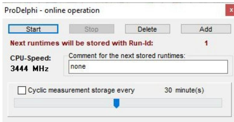
you can start and stop the time measurement. This enables you to measure only certain activities of your program. The 'Start'-button enables the measurement, the 'Stop'-button disables it. With the 'Delete'-button, all counters are set to zero. The 'Add' - button appends the actual counter values to the result file and sets the counters to zero.
