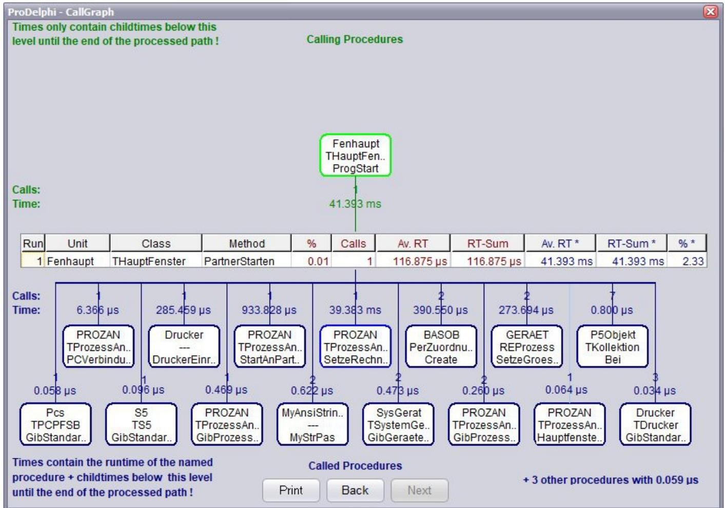
The 'Critical path' window displays the call sequence with the highest execution time beginning with the method displayed in the grid.
